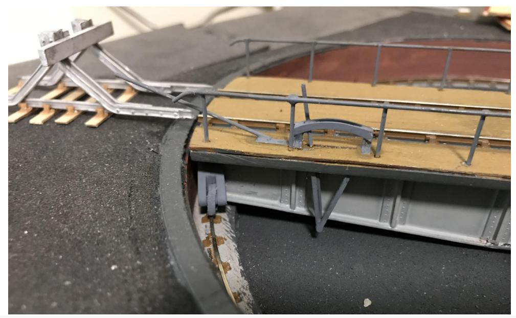
**Detail of push poles and locking lever.** Note functional rail beneath cosmetic wheel: functional in that two wipers under each end of the table pick up current from opposite halves of the circular rail.
