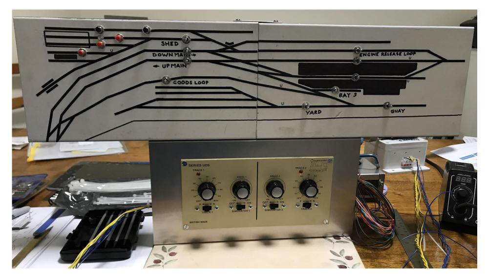
Below is the fiddle yard control box, with selection switches for which controller to power the fiddle yard sections - mainly the traverser. Tracks will be powered either by the fiddle yard controller - shown here - or the main control panel. The two control units required separate transformers - the main panel used both windings of one, and the fiddle yard use just one winding, leaving one winding free for other supplies - possibly uncoupling magnets.
