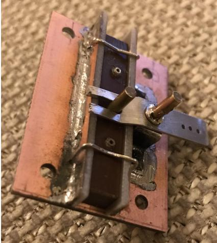
Two 1.6mm brass tubes are also mounted into the slide, but point the other way, and up through milled slots in the base, as above.
