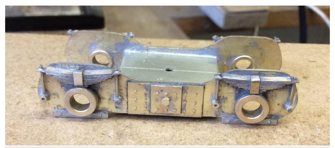
The front bogie was built up from scrap brass and n/s. Again, a frame spacer was made first, incorporating a drilled-out pivot hole for the swinging arm. Overlays were cut out, punch riveted, then soldered in place in the centre of the sideframes. Leafsprings were made from 1.5mm wide n/s strip with the correct 7 leaves each. Supporting struts are 0.6mm n/s rod and tubing. From normal viewing angles, none of the springs can be seen but I know they are there.
