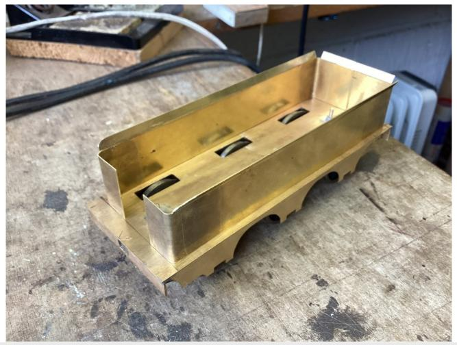
Before any brass was cut, cardboard footplate templates were again used. The most critical area was giving enough clearance for the middle and rear axles to move up within the slots. The two sideframes were then cut out and soldered in place.
