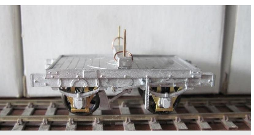
The cast parts for the brakes need some work. The lever supplied by Chris is marginally long, so I cut it and redrilled a hole for the pivot.
