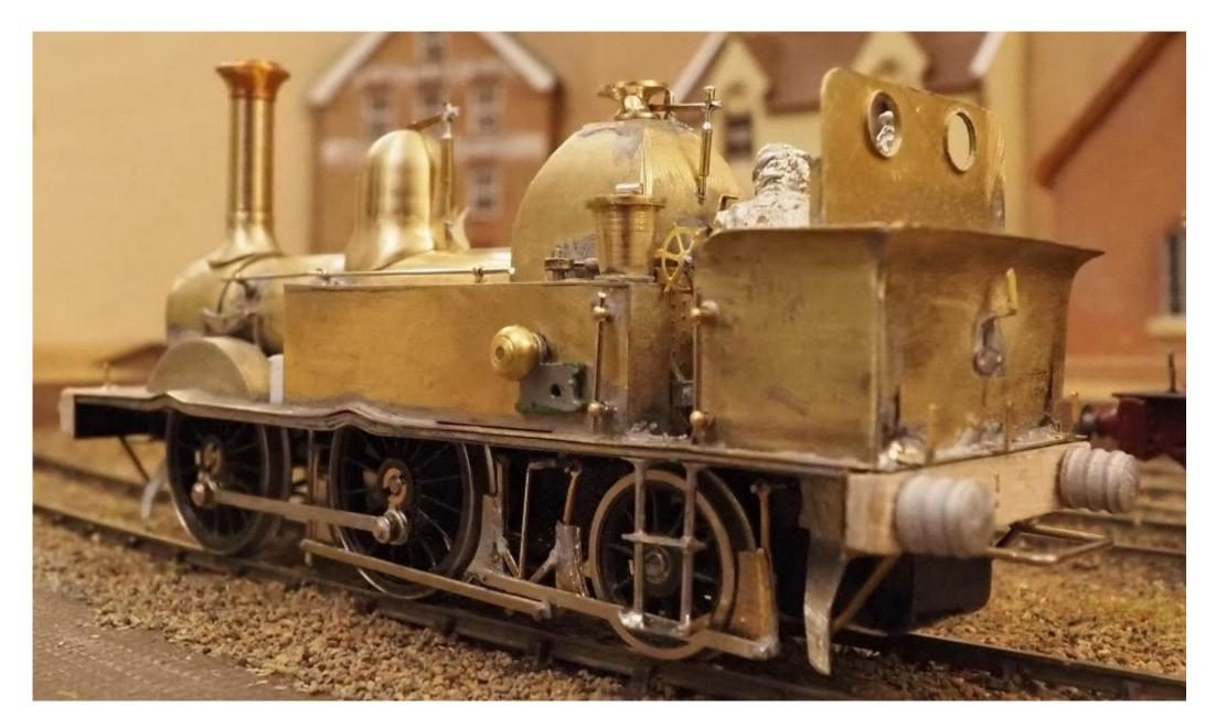
Running with the new style 1020FE iron core motor is smooth with a Gaugemaster Model W controller but erratic with the Model HH feedback controller that I am used to using with my other small loco models, all of which have Mashima motors (mostly 10 series; some 12 series).
