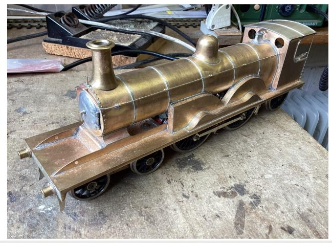
The finished locomotive barring a few incidentals such as the lubricators, Westinghouse pump, lamp irons, roof whistle and vac pipes. The most critical area to get right was a perfectly parallel boiler, followed by the four curved splasher surrounds which had to hug around the boiler. The white metal smokebox door was turned down from a much larger SR one and is fitted with a scratch made smokebox dart.
