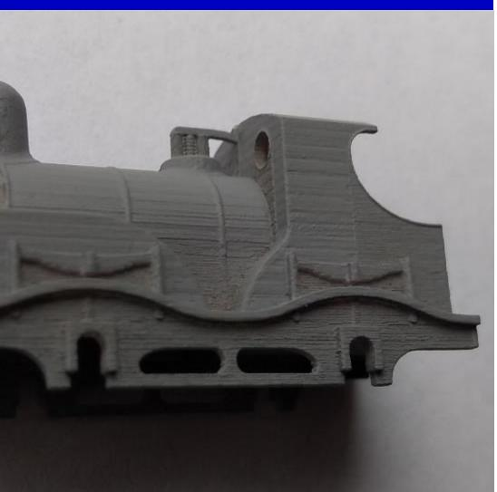
Most dimensions were very close but a lot of detail needed to go, which sanding was going to remove anyway. I removed the springs, boiler bands, dome, safety valve, smokebox door, cab roof and a portion of the outside frames. A new roof, reshaped cabsides, new dome, safety valve, footsteps, front wing plates and smokebox door were added.
