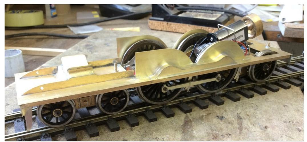
The footplate has now had side valancing (3mm x 3mm L angle) fitted, along with the headstocks, saddle sideframes, curved saddle, and guard irons, as per the drawing. Because all four drivers and coupling rods move up and down, the radii of both splashers had to be increased slightly for the maximum upward movement. Again, these areas are subtle and not noticeable. Just visible behind the rear driver is a brake hanger and shoe.
