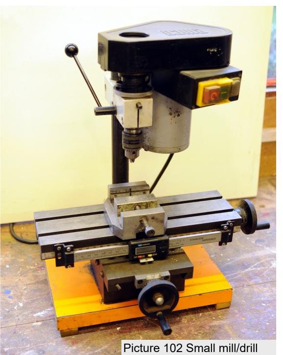
drilling and serves for what I need. A basic small drilling machine would be suitable for what most people require, although those who work in the larger scales may find a use for a bench drilling machine with a 13mm capacity chuck. When drilling through flat sheet support the material on a piece of scrap wood which will prevent damage to the table of the machine.
