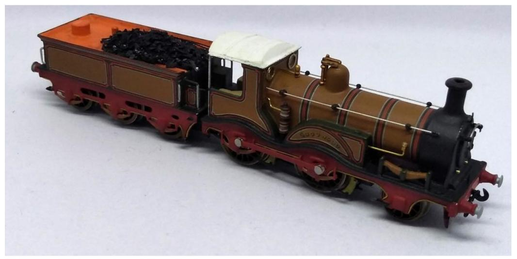
The springs posed a problem as you can't add or remove the drivers with them in place. As a result, holes were drilled in the frames for them and they are fitted afterwards and held in place with Micro Krystal Klear, so, if they need to come out, a dab of water will loosen them. As it is, the drivers are free wheeling, so shouldn't need to be removed.
