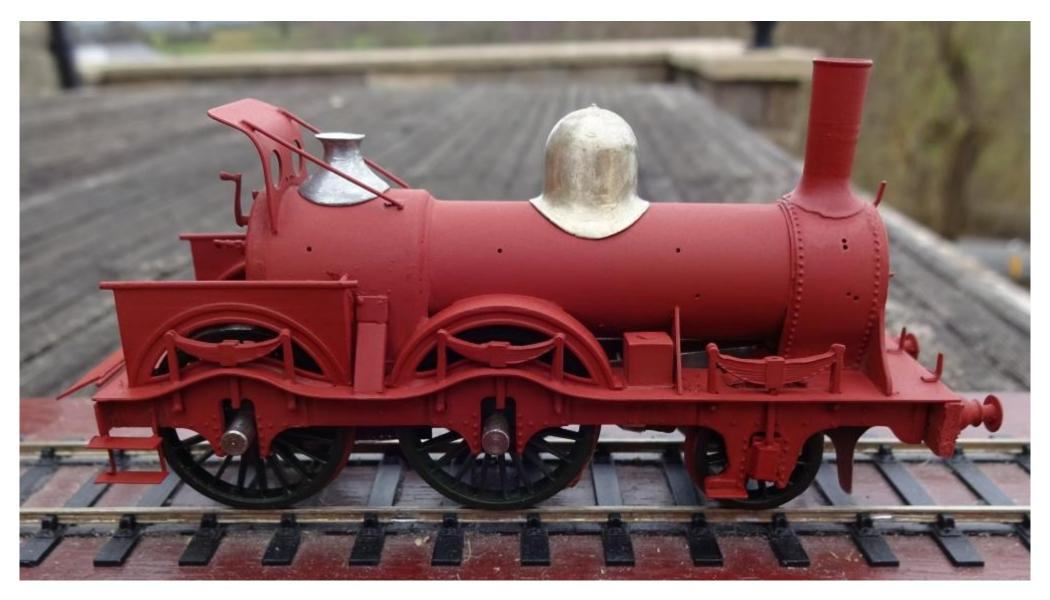
The stovepipe chimney is one of Ian MacCormac's prints. The original print is very fine and commendably thin, but caused me to worry about vulnerability. I therefore ran a coat of Araldite down the inside to give it a bit more substance, without affecting the top rim too much.
