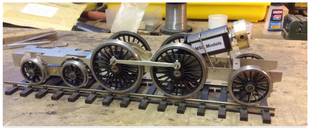
This view shows a near complete chassis after it has been fitted with the excellent MSC Models SM motor with 30:1 single reduction gearbox (<u>www.mscmodels.co.uk</u>) with flywheel and run-in in both directions. A double reduction gearbox would have been preferable but it wouldn't fit in. The single reduction gearbox still gives superb control.
