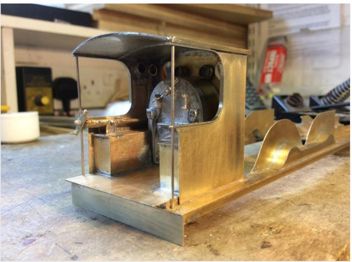
LB&SCR K Class 2-6-0 version and is not quite 100% accurate. The reversing handle can rotate. For strength, the cab roof was made from n/s sheet with 1mm x 1mm L angle rain strips. Beading strips were 1mm wide n/s strip, with 0.8mm n/s rod grab rails.
