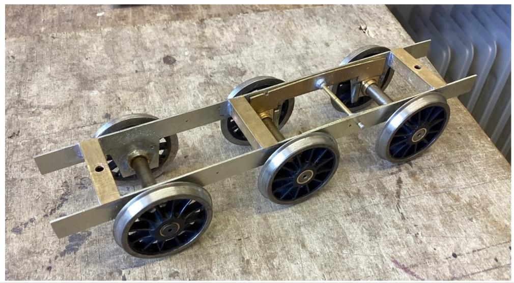
The basic frame, soldered (Carrs Speedy Solder) together, using my own  $\frac{1}{4}$ " square brass frame spacers. Each one has a lip on top, that fitted into the filed slots as shown in the previous photo.
