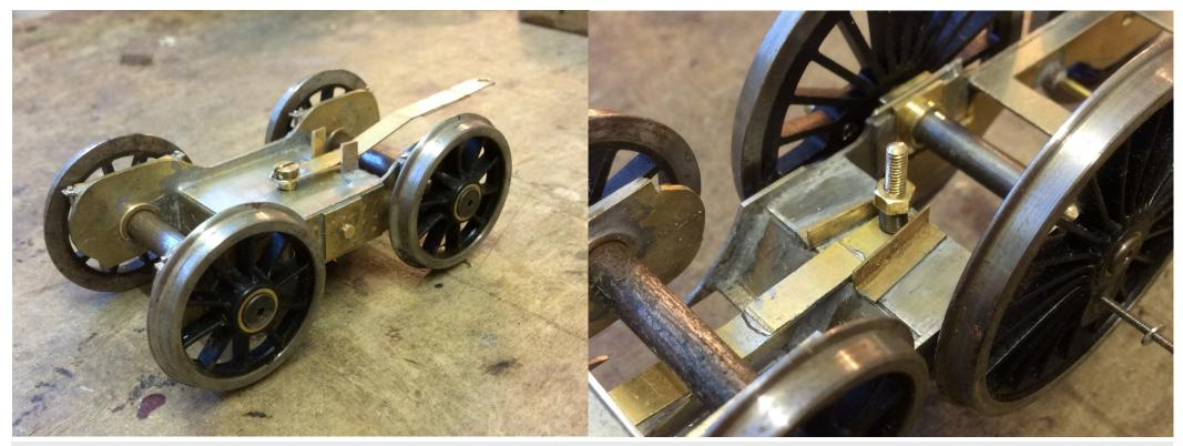
Left - The front bogie with wheels fitted. The long pivot beam is clearly visible, which gives enough downward pressure to keep it firmly on the track. Two vertical 'swing arm restrictors' can also be seen. With minute adjustment of both, the bogie has been set up to negotiate just under a minimum 6' 0" radius curve.
