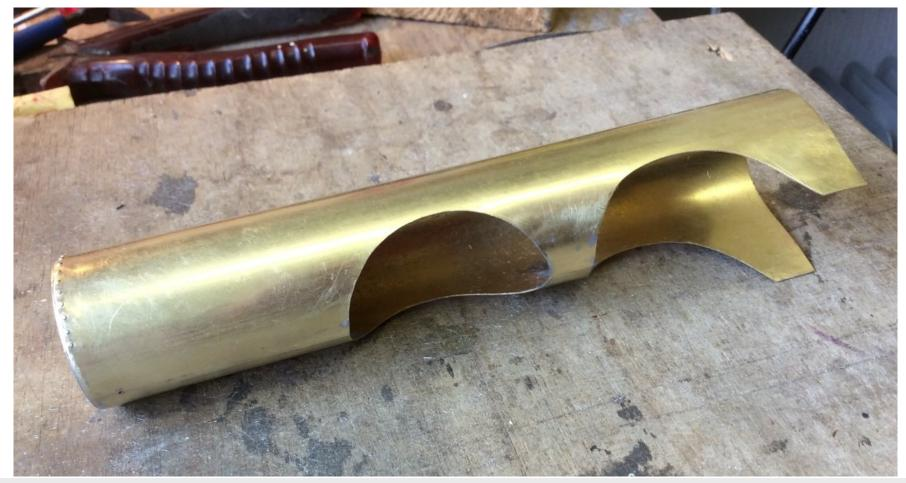
A couple of cardboard boilers were made to check wheel tread clearances. Only when I was totally happy with it was the proper boiler rolled; any mistakes would have led to a new piece of brass sheet. After rolling, a waste bit of brass was soldered on the inside of the seam. The grim task of cutting out the driver openings and filling to shape took forever. Finally, the firebox was opened out into a gentle flare. I checked numerous times that it sat level on the saddle and footplate.
