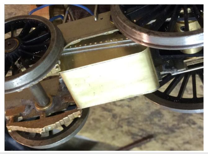
The ashpan was built up using scraps of brass and soldered as a separate slot-in unit. Being a very tight squeeze, it had to fit between the 3' 6" lost wax keeper plate leafspring castings (<u>www.lgminiatures.co.uk</u> Ref:27-042) and the rear of the gearbox. To the right, behind the rear driver, a temporary 0.7mm n/s rod keeper plate can be seen which will be substituted with a (lgminiatures Ref:27-043) lost wax compression spring casting.
