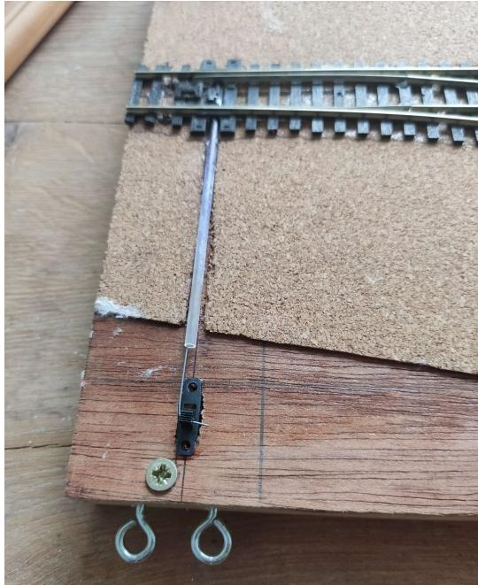
controlled by wire in tube, the tube being part of an old ballpoint pen!
