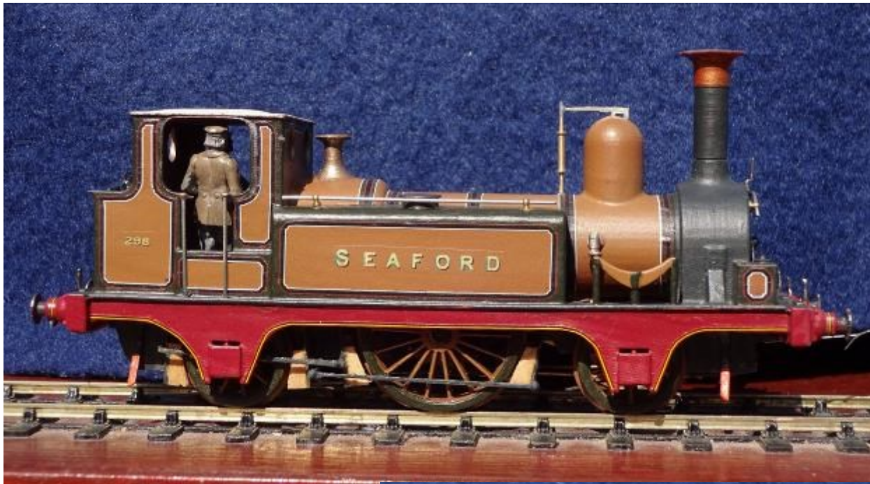
Seaford - Built in 1859 and modified in 1873 by Stroudley. Withdrawn 1879. Model from a 3D print with a scratchbuilt brass chassis.
