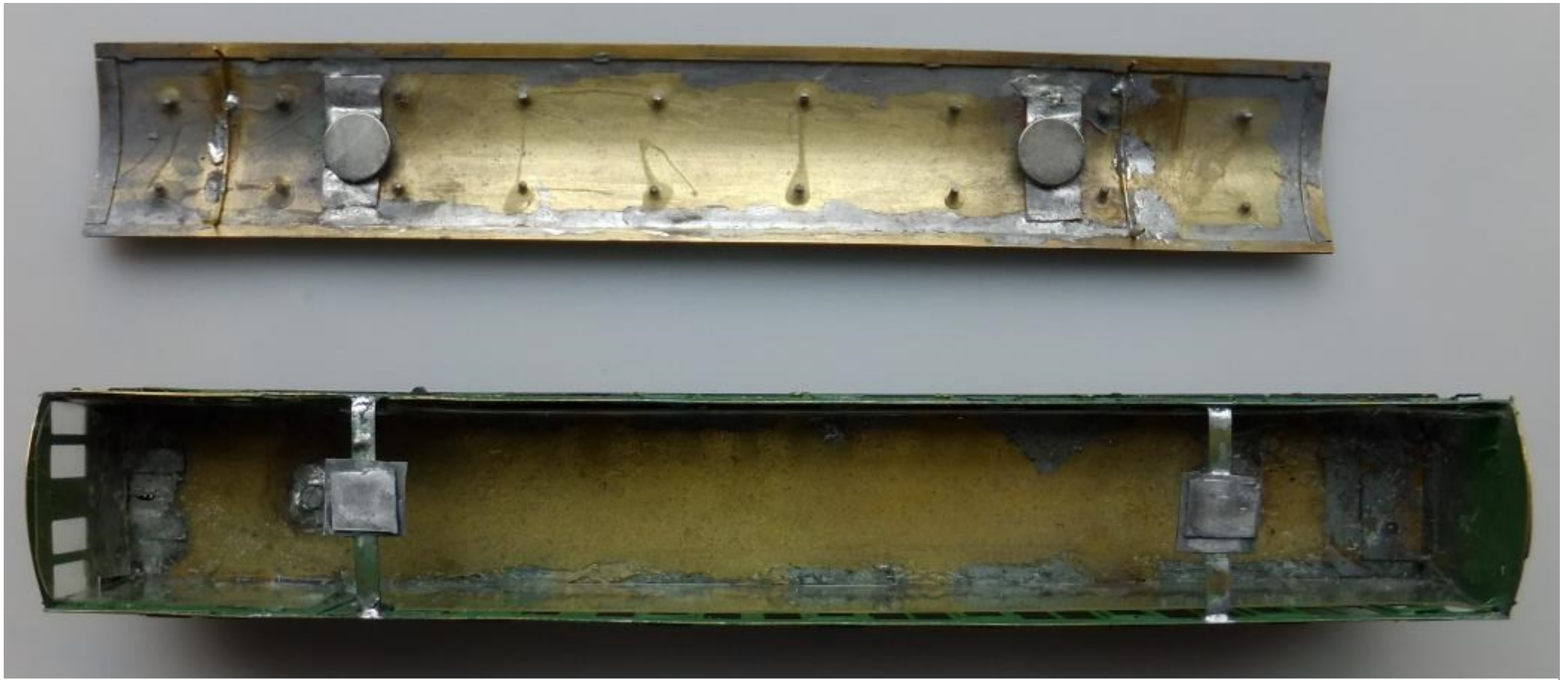
Arrangement of magnets to retain the roof.
