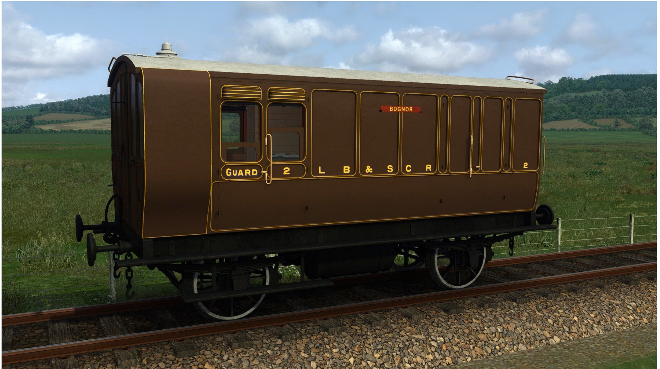
D47/222 4-wheeled luggage brake van no. 2 in umber livery of the early 1910s.
