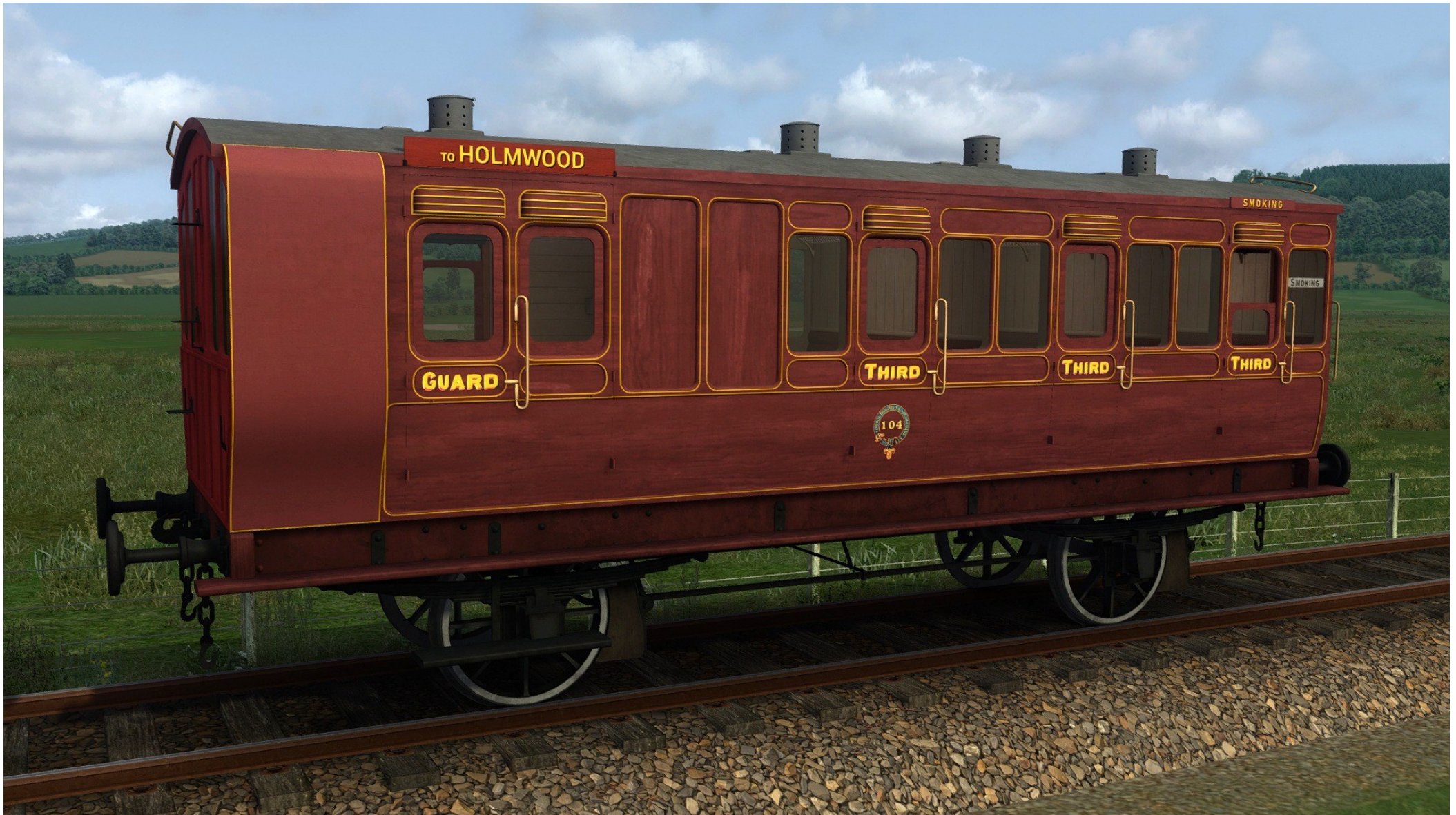
D45 Brake Third 4-wheeled brake third no. 104 in later 1870s condition, still with wooden brake blocks and oil lamps.
